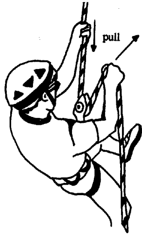
Figure 14: Releasing with weight on rope
